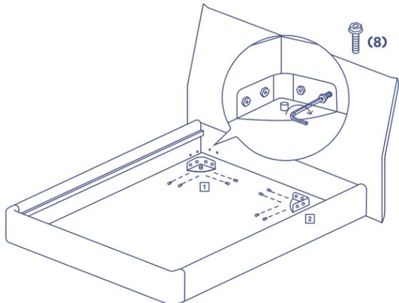
Attach the remaining two corner brackets on both sides.
