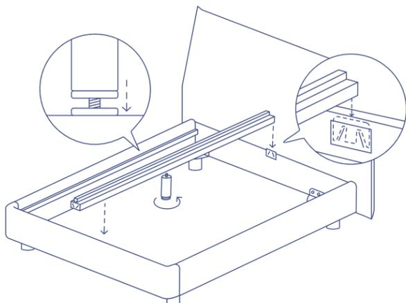
Screw center leg into the bottom of the center beam. Attach center beam onto the hitch by sliding it down into place. Unscrew leveling foot underneath center leg until it's stable on the floor.
