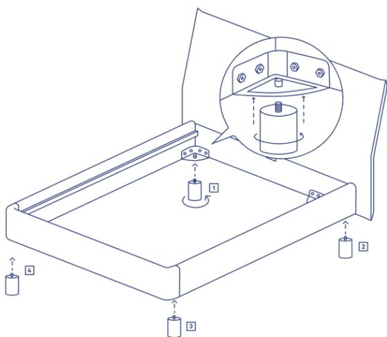
Lift up corner of bed frame and screw in a corner leg, counterclockwise. Repeat process for all 4 legs.
