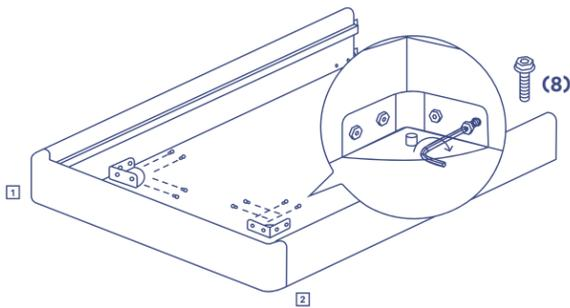
Attach a corner bracket by aligning it to the holes, then use the hex key to screw in each bolt. Fully tighten with the short end of the hex key. Repeat process for both sides.
