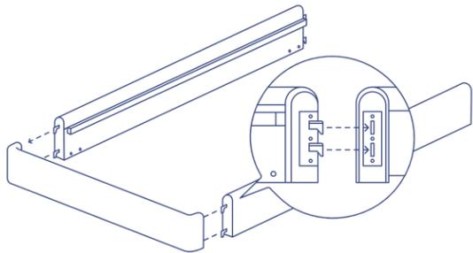
Lay foot rail on the ground. Latch the foot side of a side rail to the foot rail. Repeat process for both sides.
