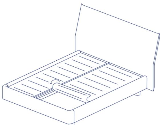
Roll out a slat pack until flat on both sides of the frame.
